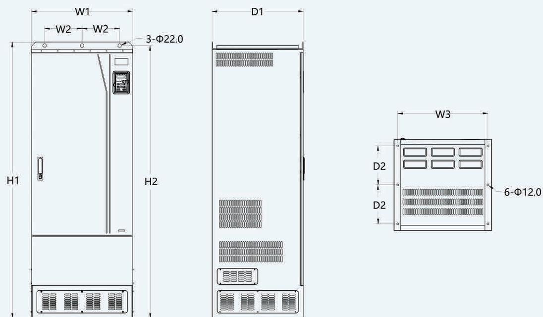
380V 355-500kW VFD floor installation diagram
