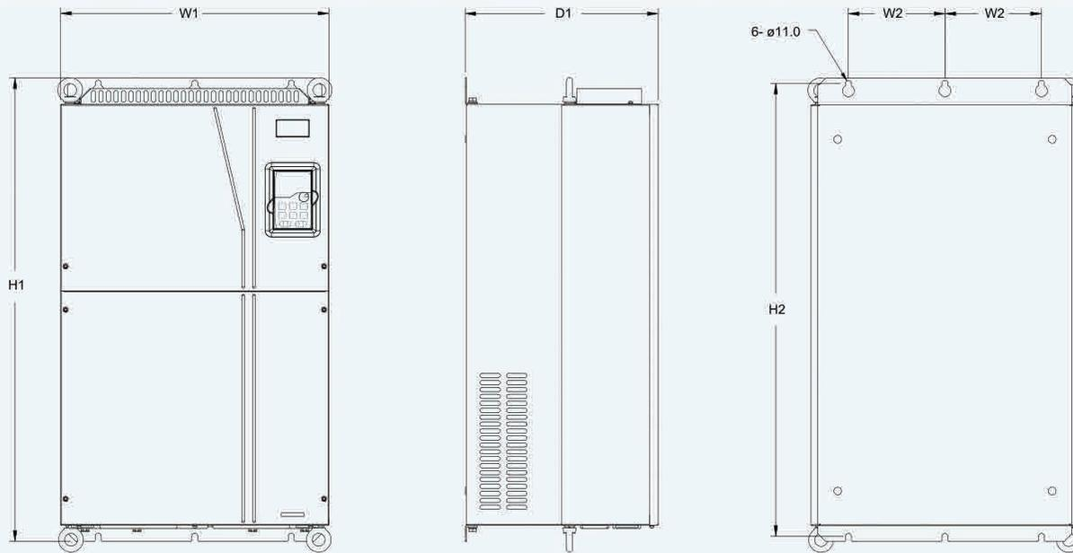
380V 132-200kW VFD wall mounting diagram
